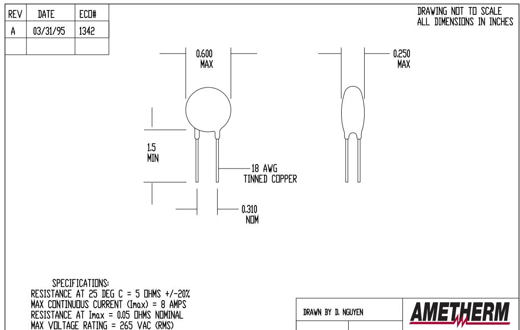
MAX CUNTINUUUS CURRENT (Imax) = 8 AMPS RESISTANCE AT Imax = 0.05 UHMS NUMINAL MAX VULTAGE RATING = 265 VAC (RMS) MAX SURGE RATING = 40 JUULES ENCAPSULATION = SILICONE RESIN MARKING = UPTIONAL LEADS = RUDAN P/N STL-209-37
